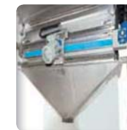
Vibrating chute allows to channel the material flow for introduction into the process downstream
